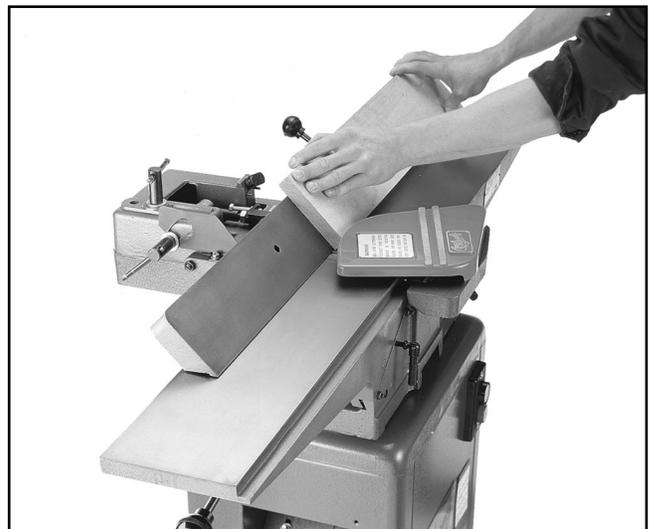
**Figure 25.** Fence position for bevel jointing.
