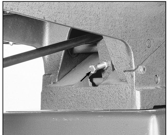
**Figure 16.** Location of the table stop bolt and jam nut.
