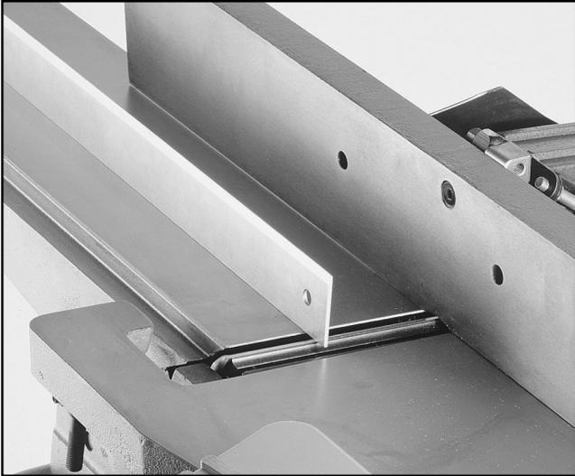
**Figure 17.** Illustrates the use of a straightedge to ensure proper outfeed adjustment.
