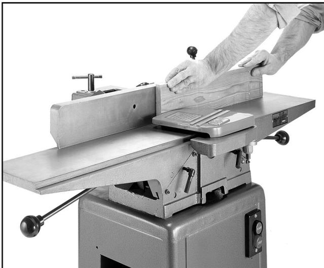
**Figure 24.** Proper operator position for edge jointing.
