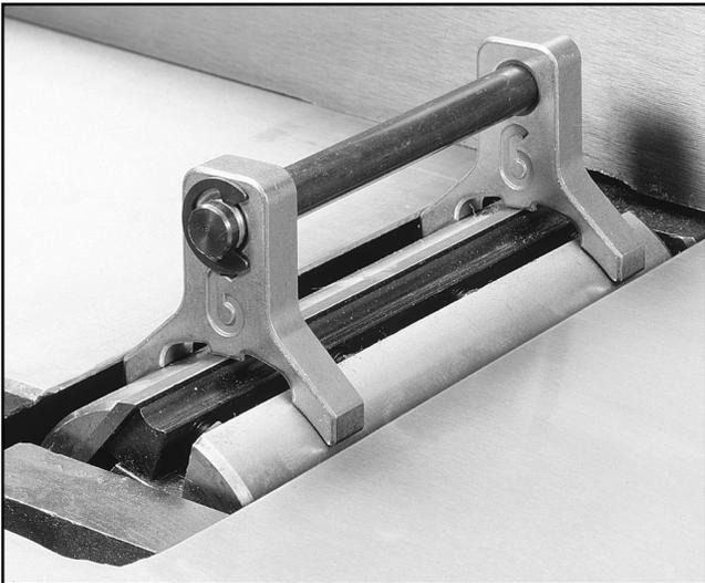
**Figure 15.** Proper positioning of knife setting jig.
