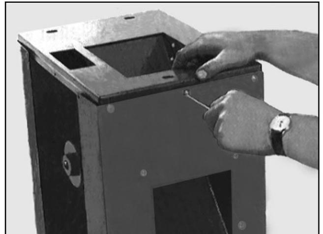
**Figure 5.** Attaching the top of the stand.
