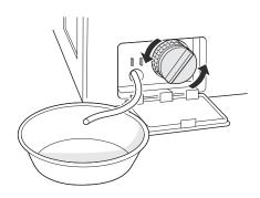
**5** Clean the pump filter and opening.
