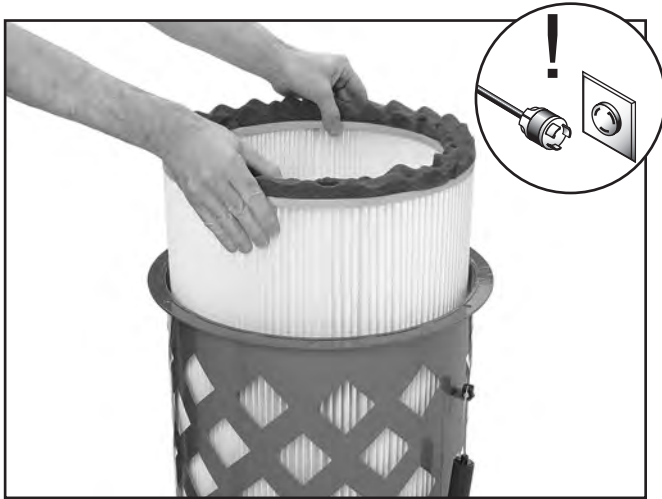
Figure 62. Removing the filter from the canister assembly.
