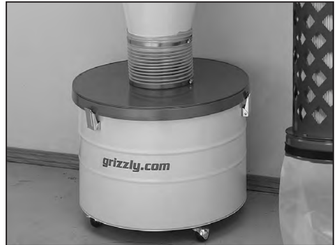
Figure 28. Drum attached to cyclone funnel with clear 9" hose.
