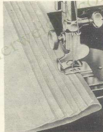
Fig. 40. Tucking with the Edge-Stitcher
