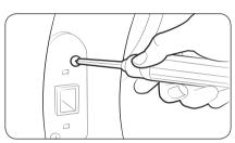
7. Remove the two screws that hold the lever holder in place, and then remove the lever holder.
