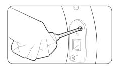
12. Push the lever holder into the cut out on the other side of the door opening. Insert screws, and then tighten as shown.
